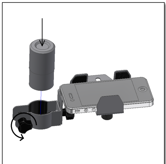
Figure 8. Release thumbscrews to insert eyepiece.
