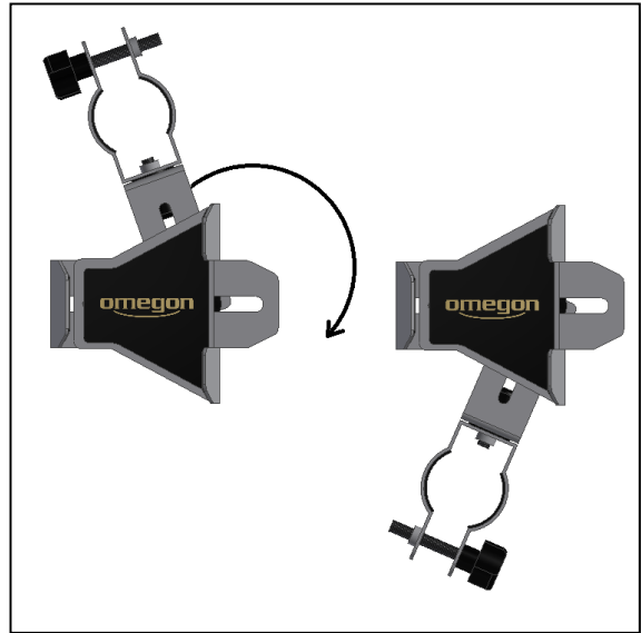
Figure 17. Rotate bracket, if necessary.
